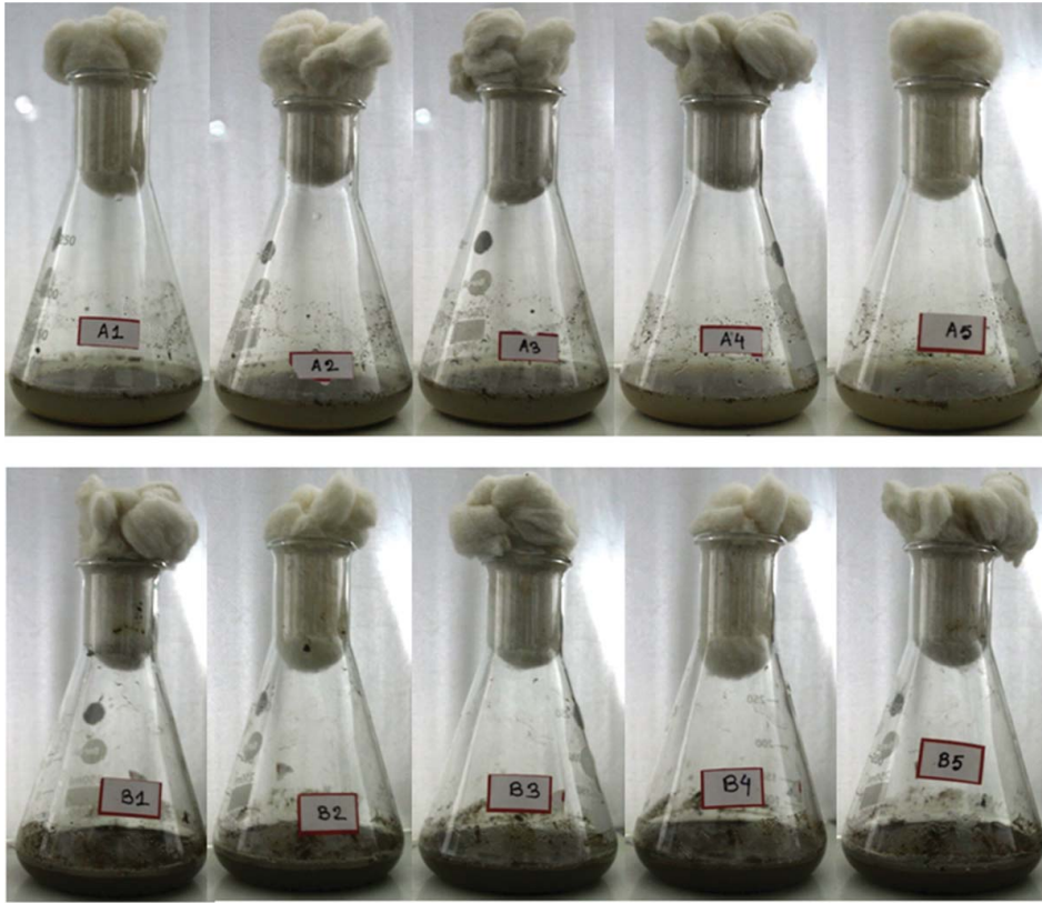
Figure 1. Photograph of a set of microcosms prepared for assessment of the impact of Arsenic on total and diazotrophic bacterial activity. In each microcosm agricultural soil was incubated in presence or absence of variable concentration of arsenic. Please see Table 1 for detail description of the microcosms.
